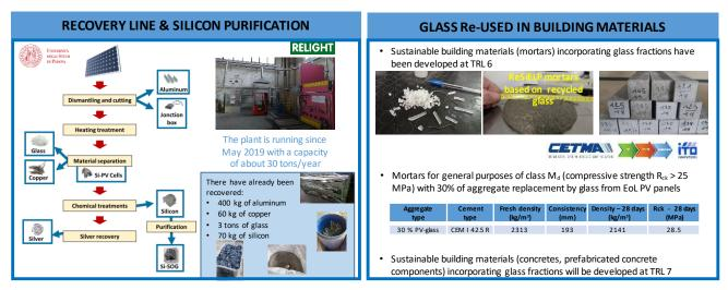
**ReSiELP** brings together <u>technologies</u> from different fields to <u>recover</u> and <u>purify critical and precious raw</u> <u>materials</u> (Si, Ag) that are present in EoL PV Si-modules. **ReSiELP** reuses by-product materials (glass, Al, Cu) in <u>an environmentally friendly</u> and <u>circular economic process</u> with a <u>product-centric zero waste approach</u>.
